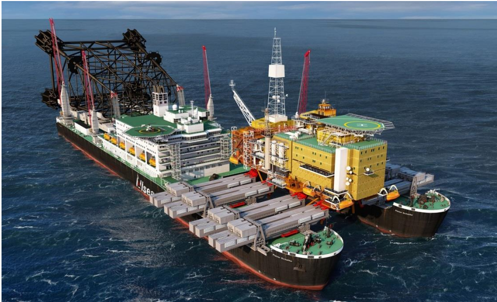
Figure 6: Allseas vessel, Pioneering Spirit , has the capacity to lift 48,000 tonnes at a time. Here it is shown with platform topsides sitting on deck (Allseas 2016)
