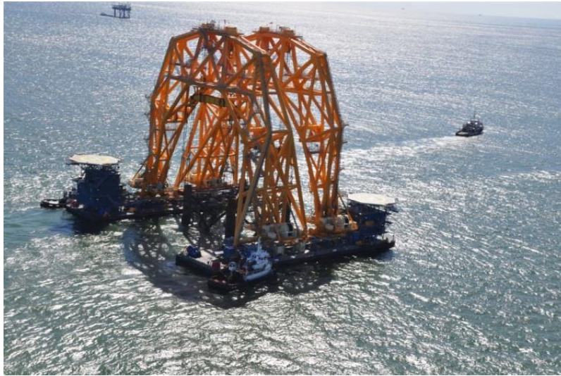
Figure 5 - The VB 10,000 lift system in operation (Wikimedia Commons 2016)
