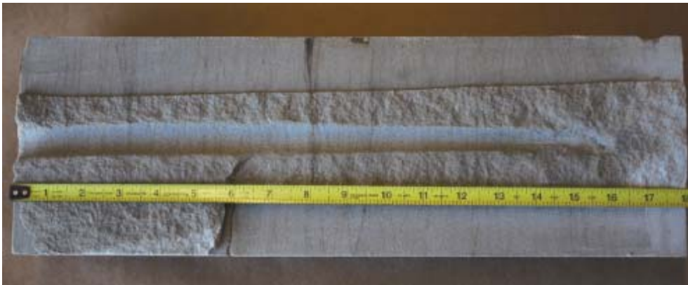
Image 11 - example of a perforation charge into sandstone
