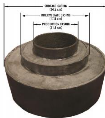
Image 3 Multiple Pipe Casings and Cementation:
